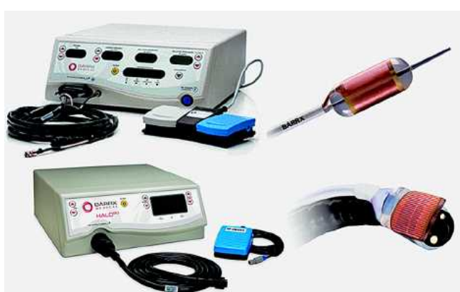
Fig. 1 The HALO system for stepwise circumferential and focal radiofrequency ablation (RFA). Upper left: The HALO 360 generator with integrated pressure:volume system, used to inflate the sizing and ablation catheters, to calculate esophageal inner diameter, and to deliver radiofrequency energy to the ablation catheter. Upper right: The HALO 360+ ablation catheter. Lower left: The HALO 90 energy generator for delivery of radiofrequency energy. Lower right: The HALO 90 catheter fitted on the tip of an endoscope, without impairing the endoscopic view or function. Reproduced with permission from www.endosurgery.eu.
